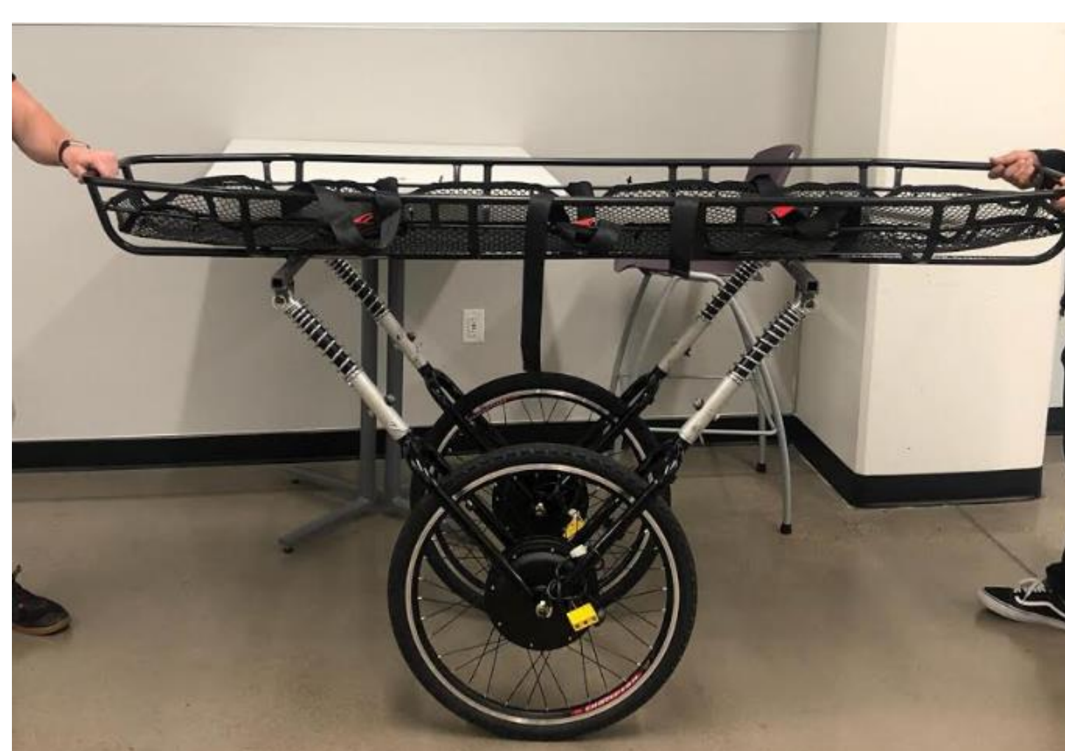
Figure 1.4: Powered litter alpha prototype build.
