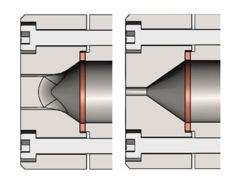
The circular die was designed using the appropriate diameter to account for the shrinkage of the material as well as other factors in order to extrude a circular filament having a diameter of 1.75mm. The rectangle extrusion shape was designed with the goal of producing a rectangular cross section of 8mm by 3mm. The design of the die assembly also allows for the fabrication of additional die geometries without the need to replace the entire end of the barrel.
