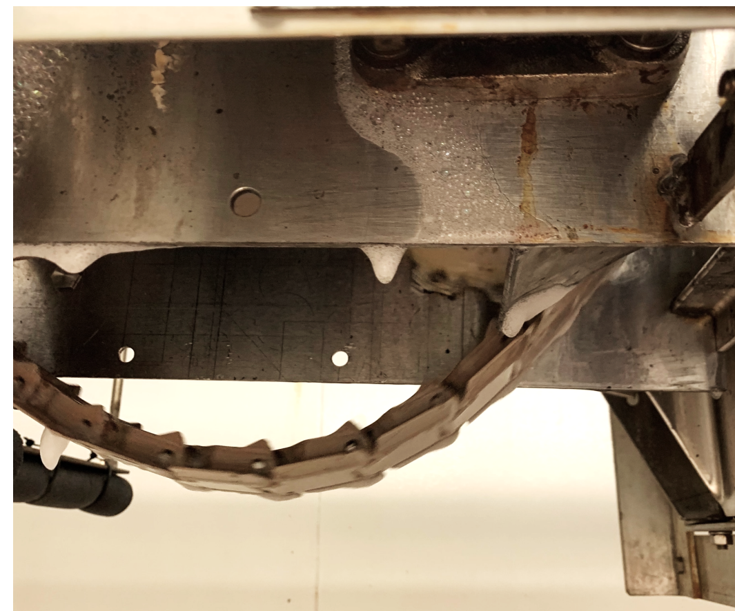
This is one section of the conveyor belt that the automated conveyor cleaning system would attach to.
